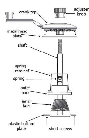
DO NOT fully tighten the adjuster knob and force the handle or you may damage the grinder burrs.
